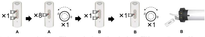
Press A remote UP and DOWN buttons simultaneously.
