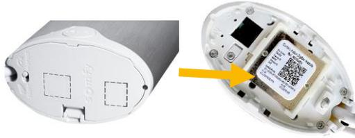
Insert the Glydea Ultra Zigbee module into the slot.
