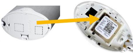
Insert the Glydea Ultra Zigbee module into the slot.
