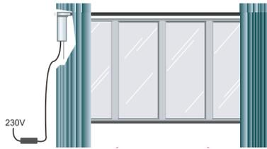
Plug the motor into mains power.
